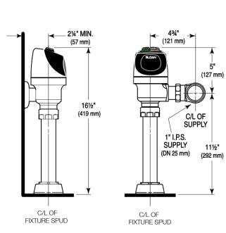
ALTERNATE ADA INSTALLATION Lower water supply rough-in to 10" (254 mm) and mount grab bar at the 36" (914 mm) maximum allowed height (top of grab bar at 36").
